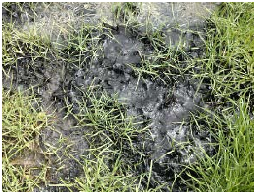
Figure 5.5. Surfacing effluent is a symptom of septic system failure that can be caused by several factors such as poor soil suitability, age of the system, or overloading. Photo courtesy of FirstCallSeptic.com.
